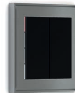
E12 - 4-fold pushbutton and room thermostat - 2 rectangular vertical rockers. Rockers: finishing plastic, black colour. Frame and plate: finishing brushed metal, titanium colour, red/white LED. Dimensions: mm 86 x 86 x 8
