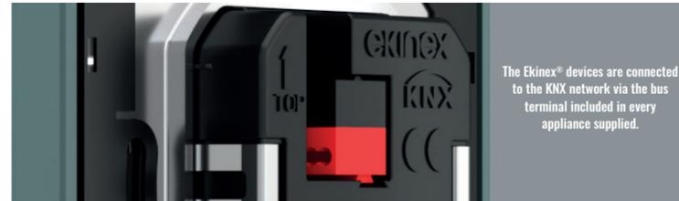
The Ekinex® devices are connected to the KNX network via the bus terminal included in every appliance supplied.
